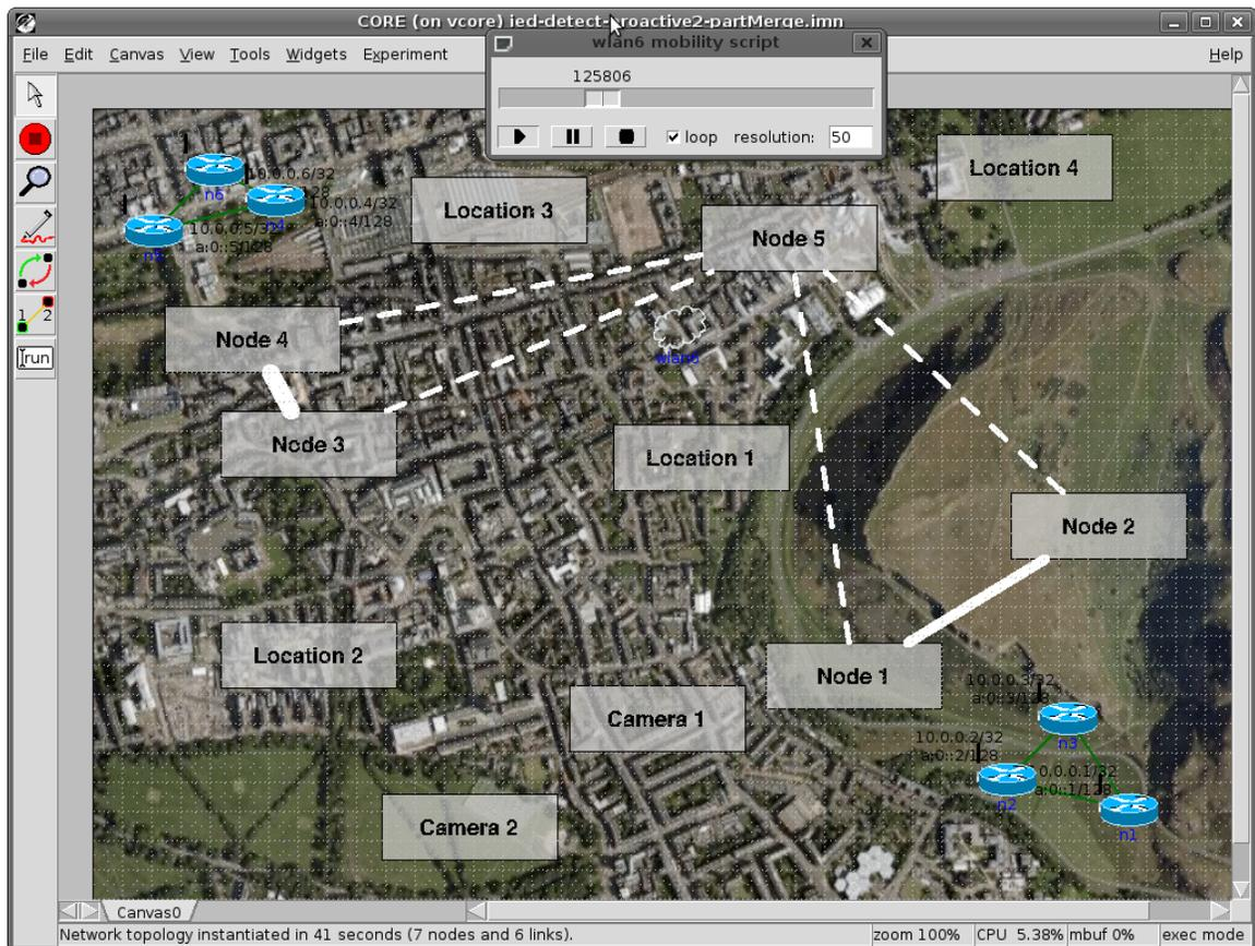
Figure 5.7: Screenshot of the partition/merge mobility model running in CORE. The blue circles are the CORE hosts, the white rectangles show the starting positions.
